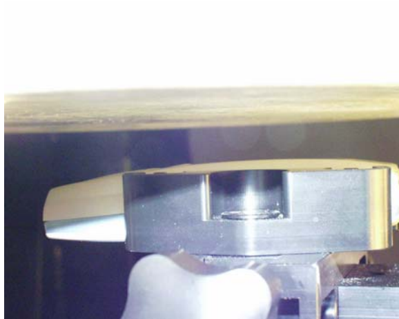
Back part of the phone 15mm away from the Flat Phantom
