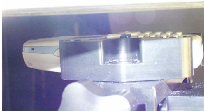
Front part of the phone 15mm away from the Flat Phantom
