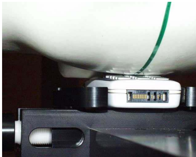
Device position against the head: Cheek (touch) phone position
