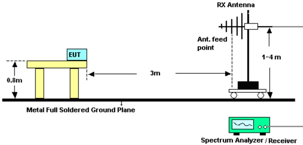
For radiated emissions from 1GHz to 18GHz
