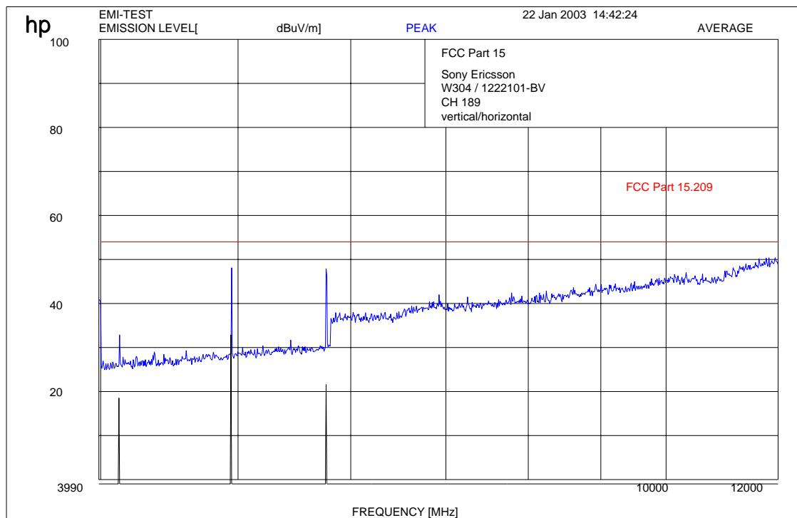
**$f < 1 \text{ GHz}$  : RBW/VBW: 100 kHz** **$f \geq 1 \text{ GHz}$  : RBW/VBW 1 MHz****Carrier suppressed with a rejection filter**
