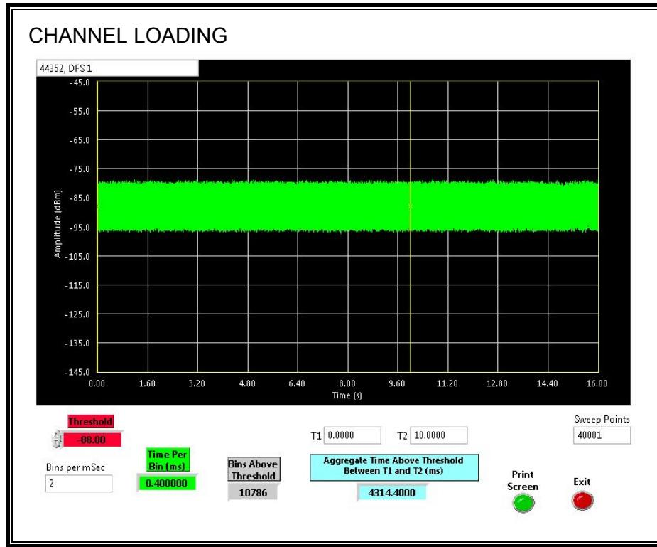
The level of traffic loading on the channel by the EUT is 43.144%
