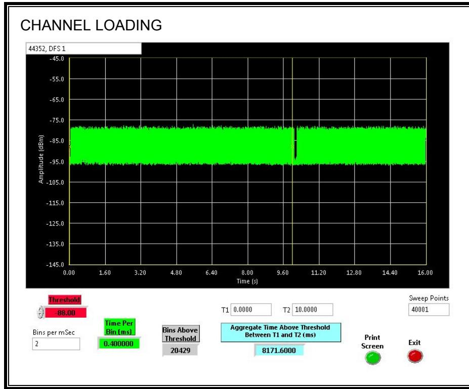
The level of traffic loading on the channel by the EUT is 81.716%.
