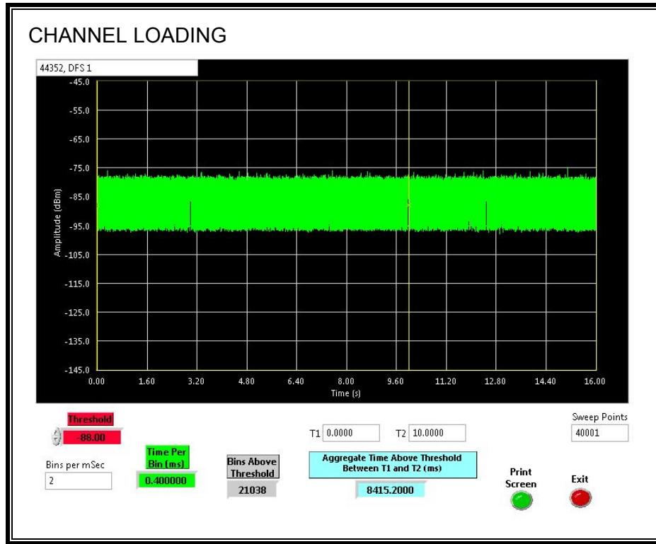
The level of traffic loading on the channel by the EUT is 84.152%.
