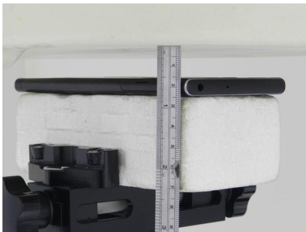
Back, Test Separation 15 mm
