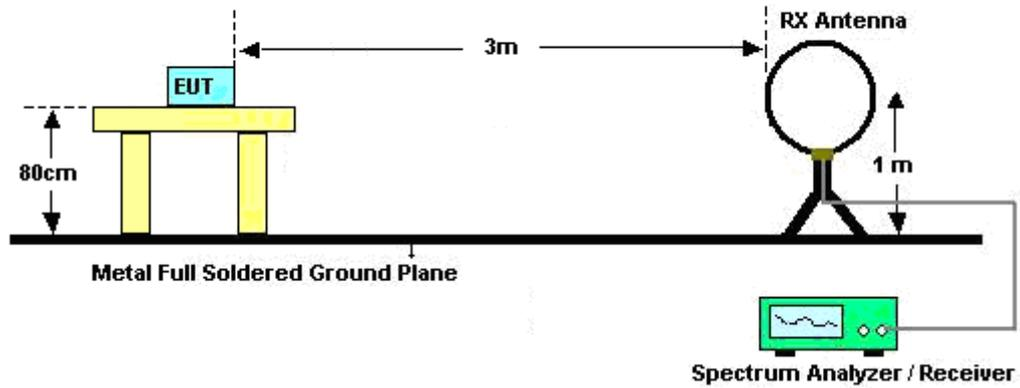
For radiated emissions from 30MHz to 1GHz
