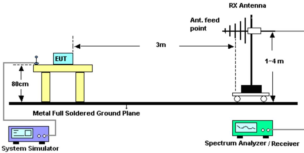
For radiated test above 1GHz
