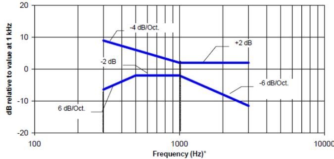
NOTE—The frequency response is between 300 Hz and 3000 Hz.
