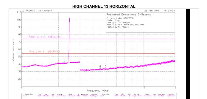
Note: Emission was scanned up to 26GHz; No emissions were detected above the noise floor which was at least 20dB below the specification limit.
