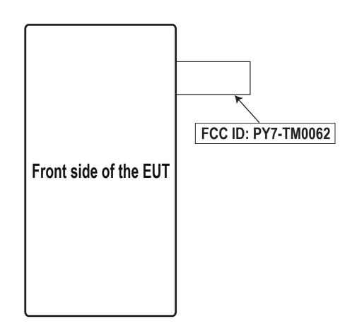
The FCC ID is not on the exterior of the device but labelling meets the conditions allowed in KDB 784748 for the label to be placed in a user accessible area:
