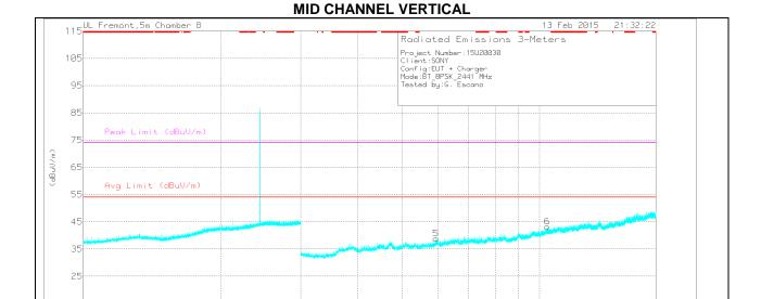
Note: Emission was scanned up to 26GHz; No emissions were detected above the noise floor which was at least 20dB below the specification limit.
