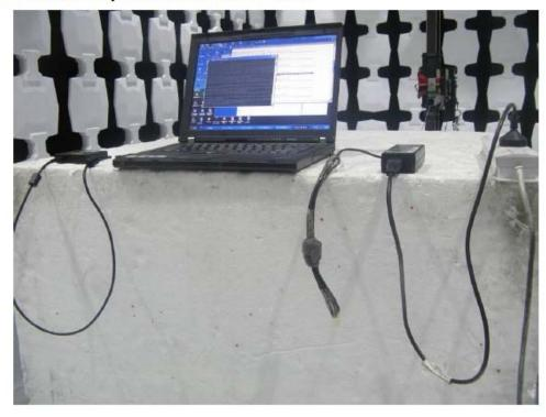
Layout of AC Powerline Conducted Emission
