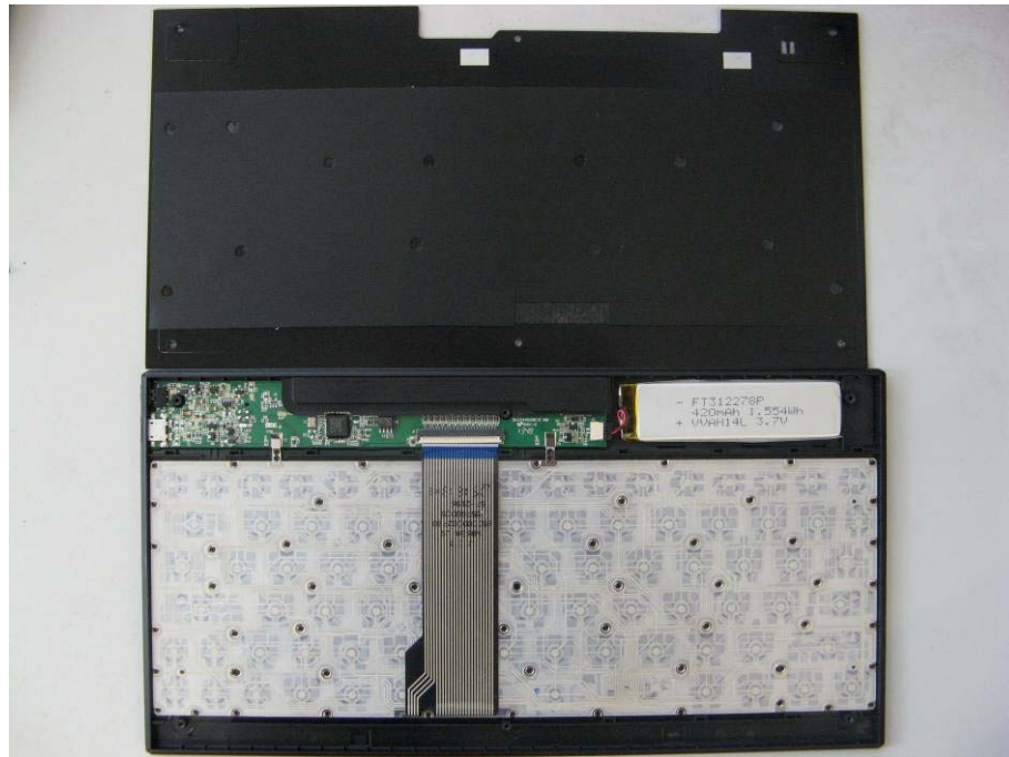
Bluetooth Keyboard Disassembly and Inbuilt Battery
