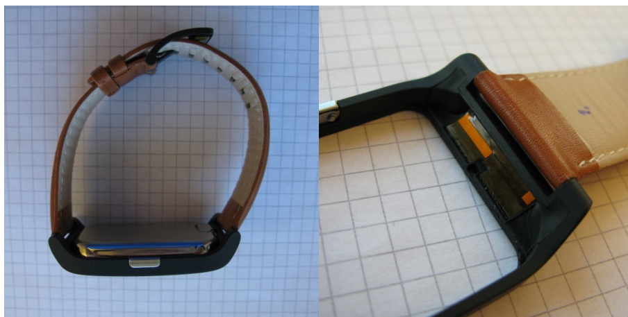
RD-0090 with carrier and band (left) and detail of the FPC film (right)
