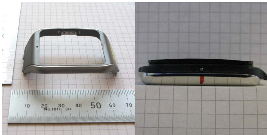
Detail of the on/off button outer part (left) and location of the button on the module (right)
