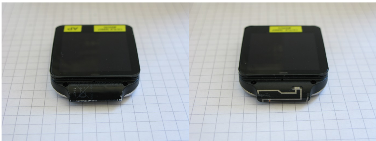
Illustration of the location of the WLAN/BT antenna (exposed on right)
