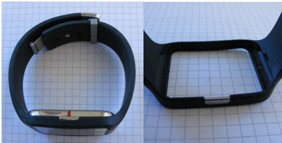
'Classic' type strap/carrier with module (left) and without module (right)
