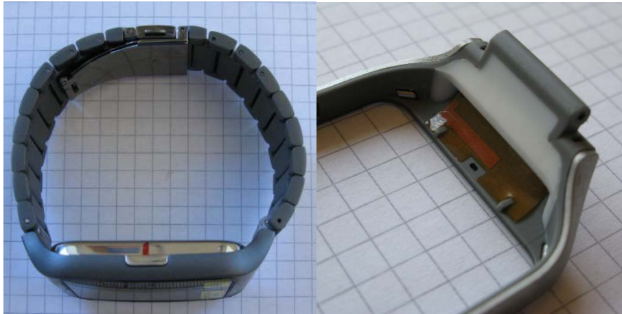
‘Metal’ type strap/carrier with module (left) and detail of the FPC film (right)
