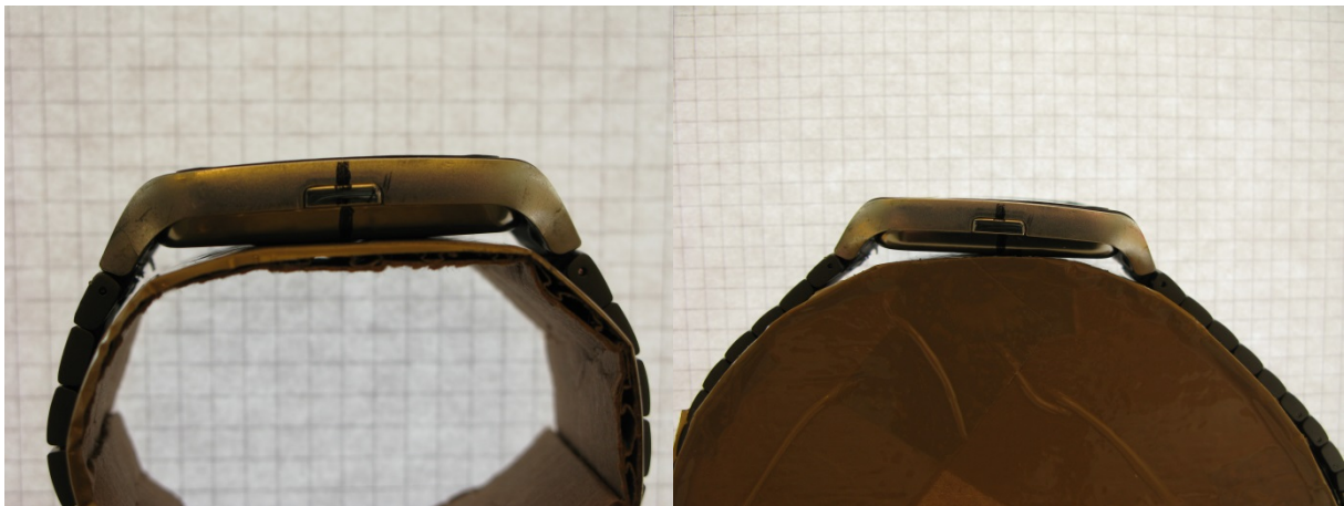
Comparison of gaps for 'Metal' type for arm (left) and phantom neck region (right)
