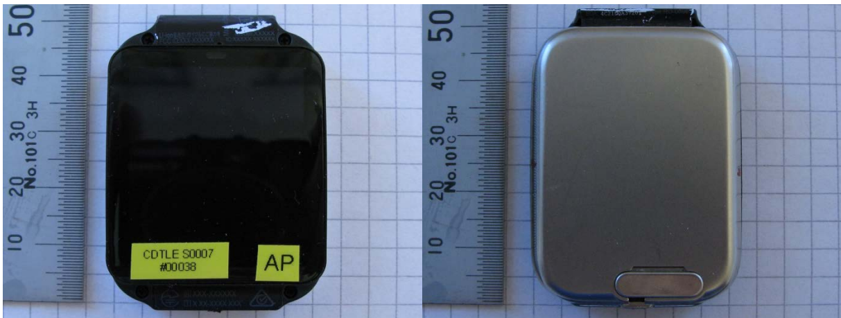
Front and rear views of the module (covered USB connector visible on rear of device to right)
