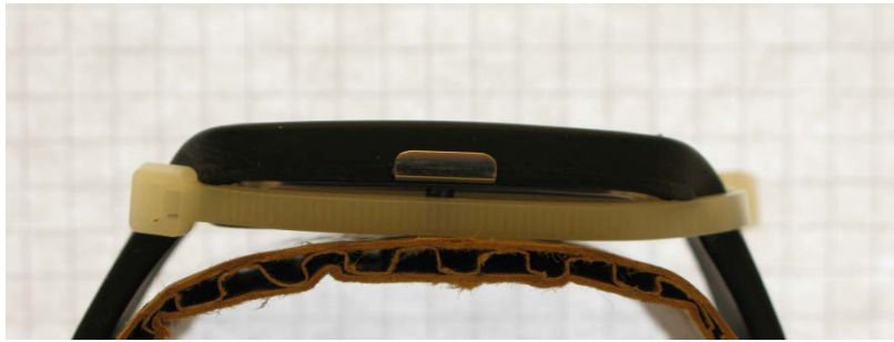
Cable Ties used to prevent distortion of the carrier for 'Classic' type
