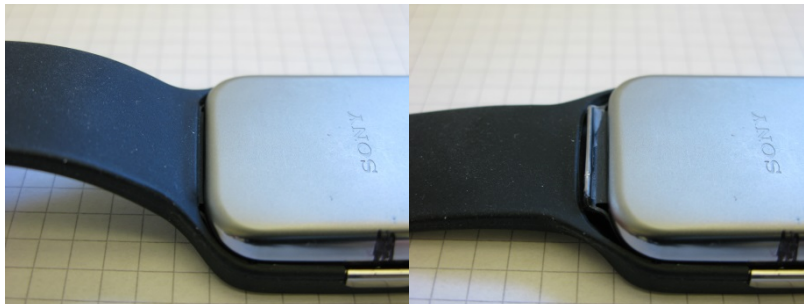
'Classic' type showing distortion to carrier if the strap is bent too far.
