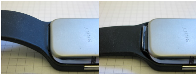
'Classic' type showing distortion to carrier if the strap is bent too far.
