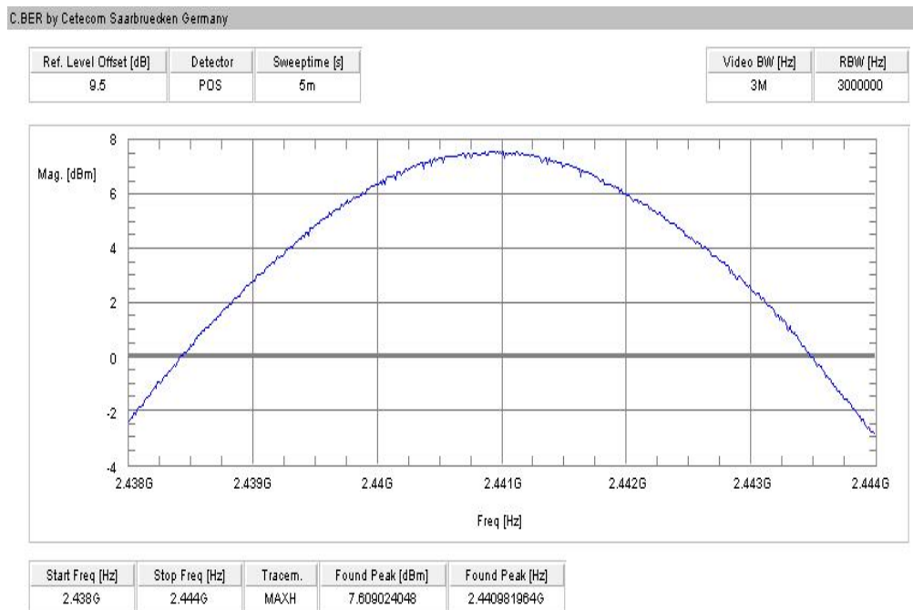
Plot 8: middle channel – 2441 MHz, 8 DPSK modulation
