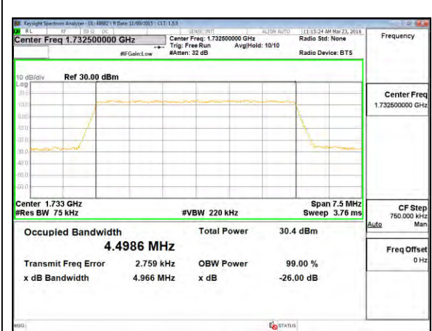
LTE B4 5MHz 16QAM Middle Channel
