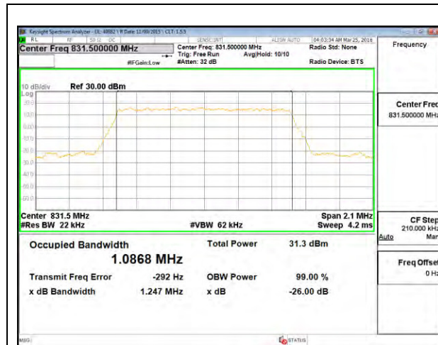
LTE B26 1.4MHz QPSK Middle Channel
