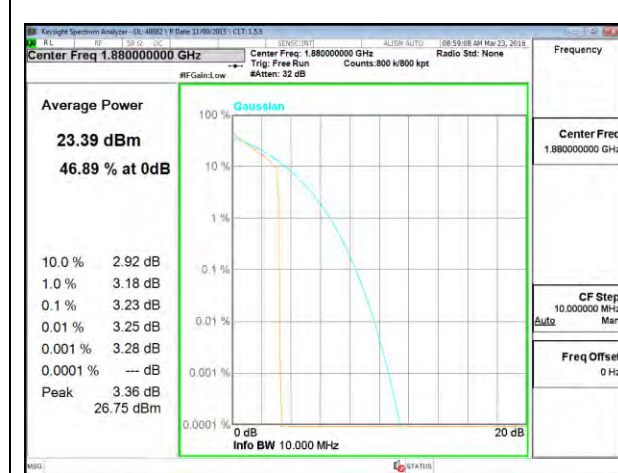
LTE B2 15MHz QPSK Middle Channel
