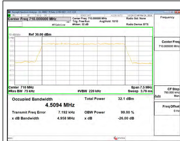
LTE B17 5MHz QPSK Middle Channel
