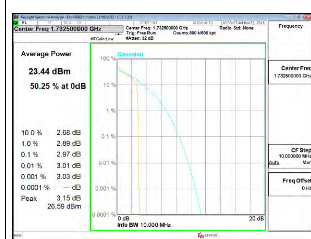
LTE B4 15MHz QPSK Middle Channel
