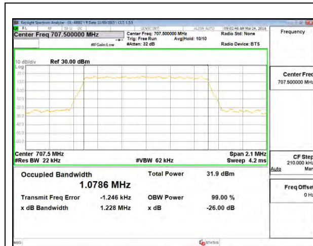
LTE B12 1.4MHz QPSK Middle Channel
