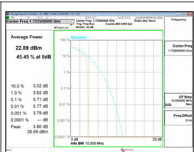
LTE B4 10MHz 16QAM Middle Channel
