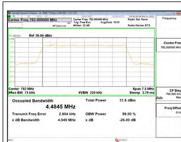
LTE B13 5MHz QPSK Middle Channel
