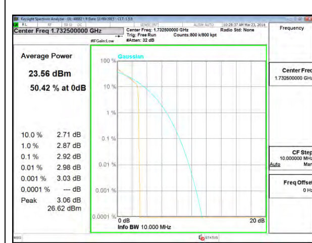
LTE B4 3MHz QPSK Middle Channel
