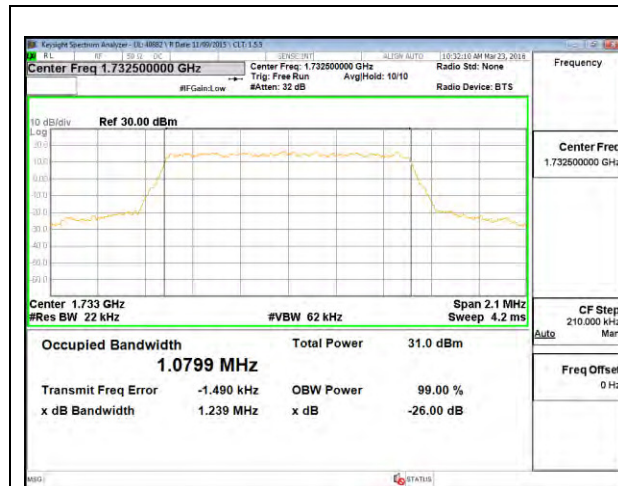
LTE B4 1.4MHz QPSK Middle Channel
