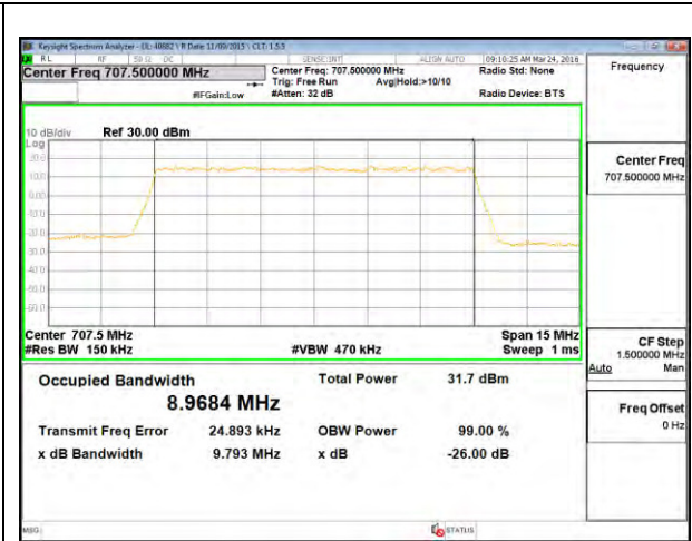
LTE B12 10MHz 16QAM Middle Channel
