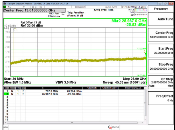
LTE B17 5MHz 16QAM Middle Channel
