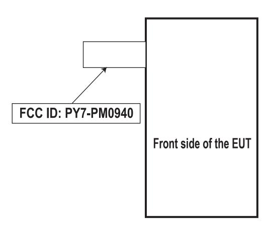
The FCC ID is not on the exterior of the device but labelling meets the conditions allowed in KDB 784748 for the label to be placed in a user accessible area:
