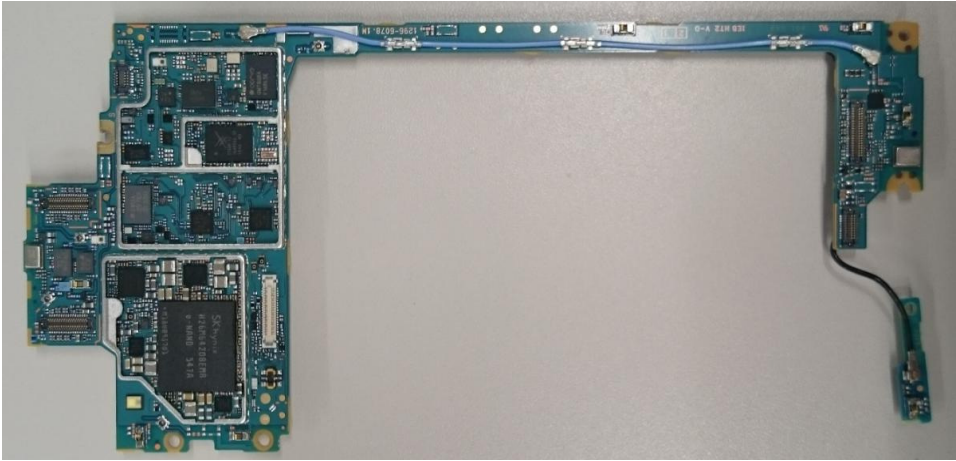
Internal PWB without Shield cases (Front side)
