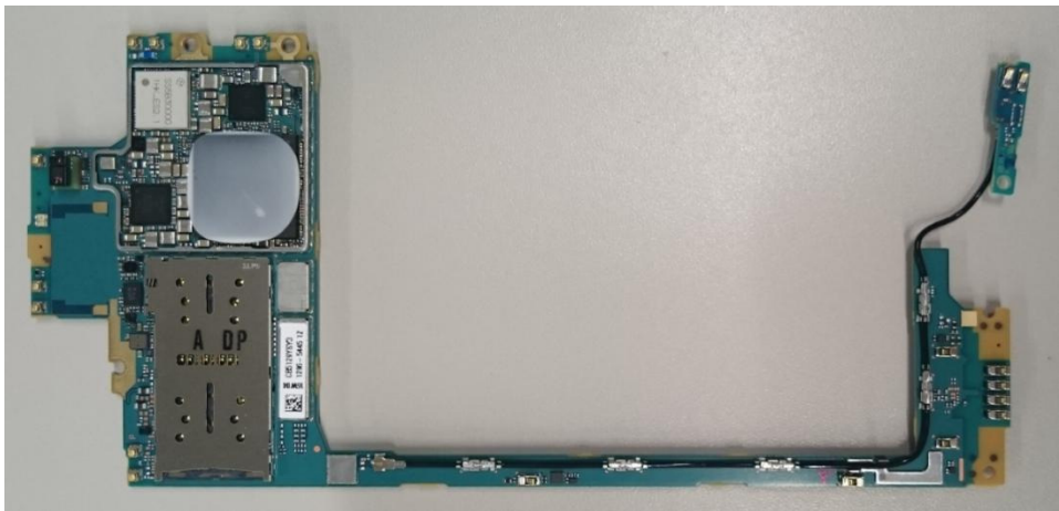
Internal PWB without Shield cases (Rear side)
