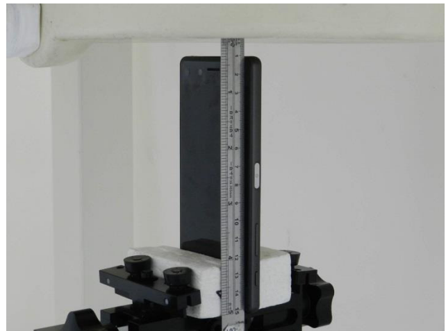
Top Side, Test Separation 10 mm
