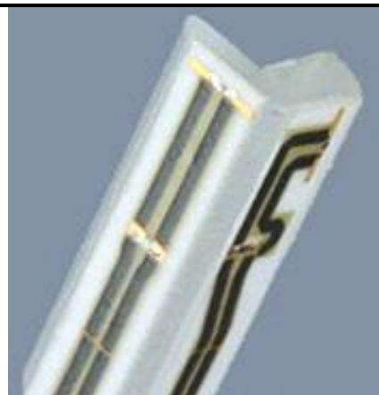
Fig 5.2 Photo of E-field Probe
