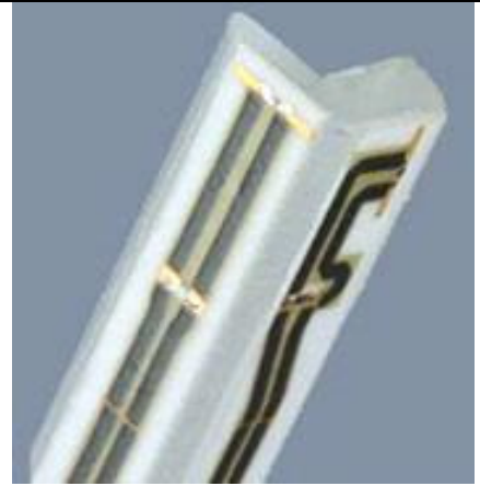
Fig 5.2 Photo of E-field Probe
