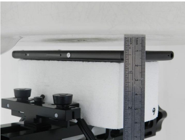
Front, Test Separation 10 mm
