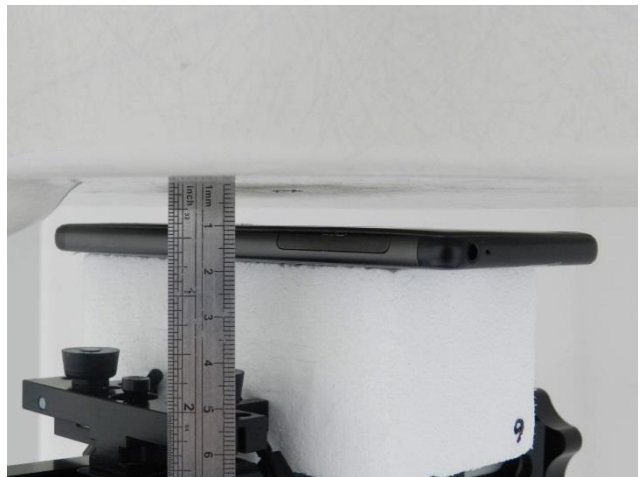
Back, Test Separation 10 mm
