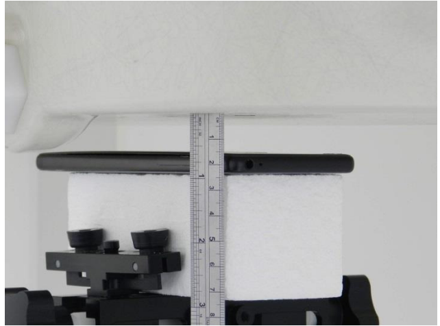
Back, Test Separation 15 mm
