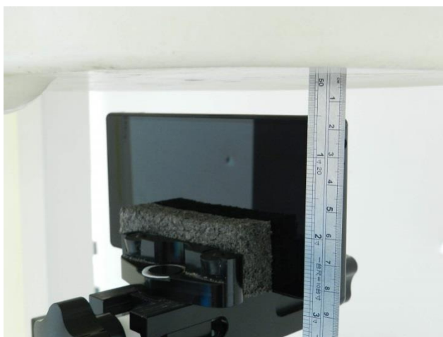
Left Side, Test Separation 10 mm
