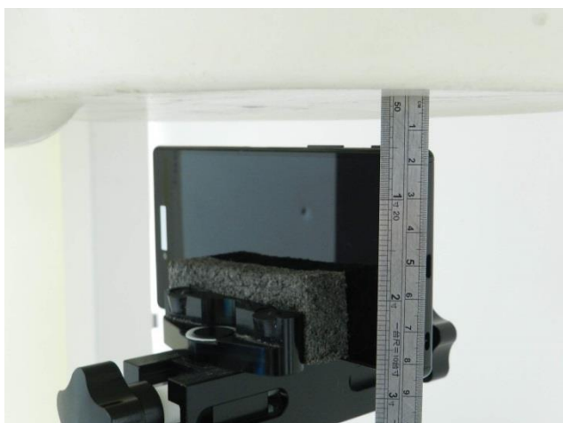
Right Side, Test Separation 10 mm
