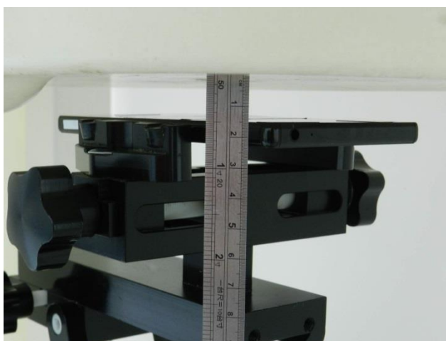
Back, Test Separation 15 mm
