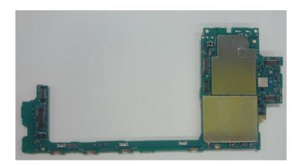
Internal PWB with Shield cases (Rear-side)
