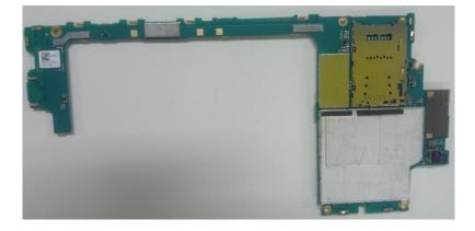
Internal PWB with Shield cases (Front-side)
