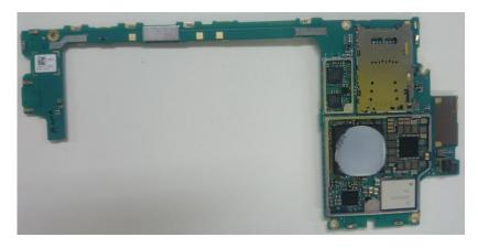
Internal PWB without Shield cases (Front-side)
