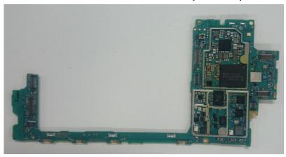
Internal PWB without Shield cases (Rear-side)
