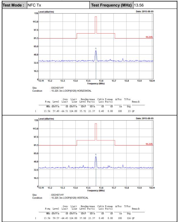
C.1 Test Result of Field Strength of Fundamental Emissions
