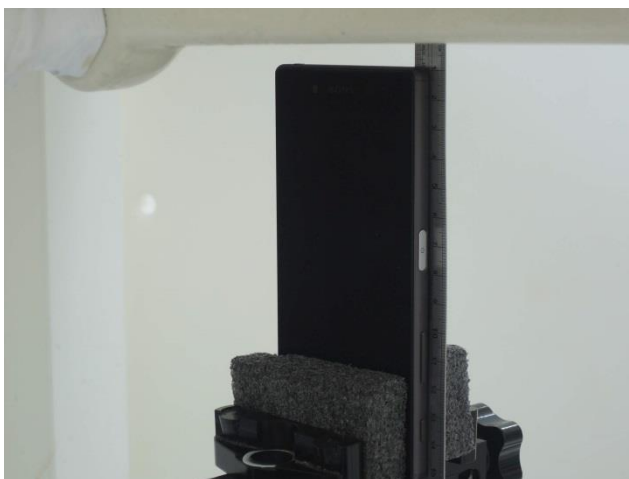
Top Side, Test Separation 10 mm
