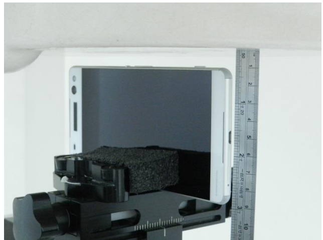
Right Side, Test Separation 10 mm
