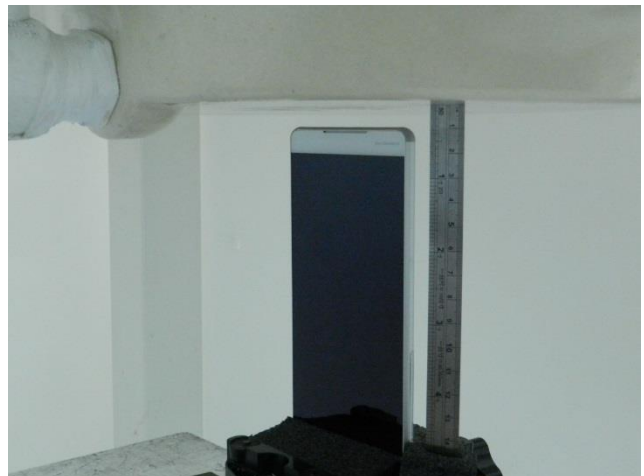
Bottom Side, Test Separation 10 mm
