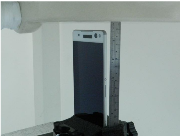
Top Side, Test Separation 10 mm
