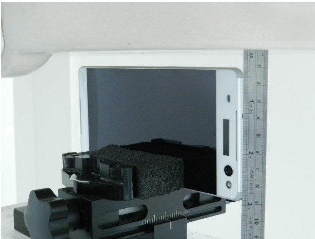
Left Side, Test Separation 10 mm
