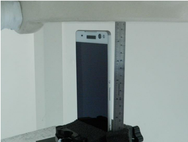
Top Side, Test Separation 10 mm
