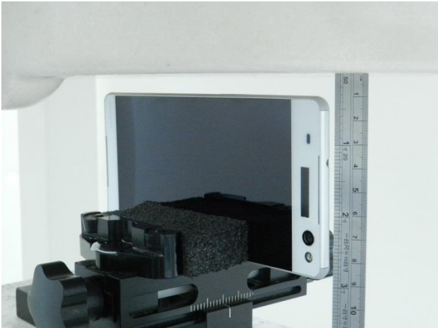
Left Side, Test Separation 10 mm
