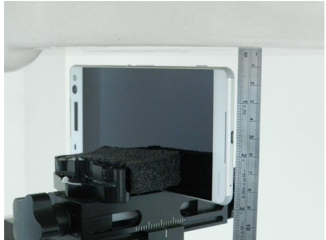
Right Side, Test Separation 10 mm
