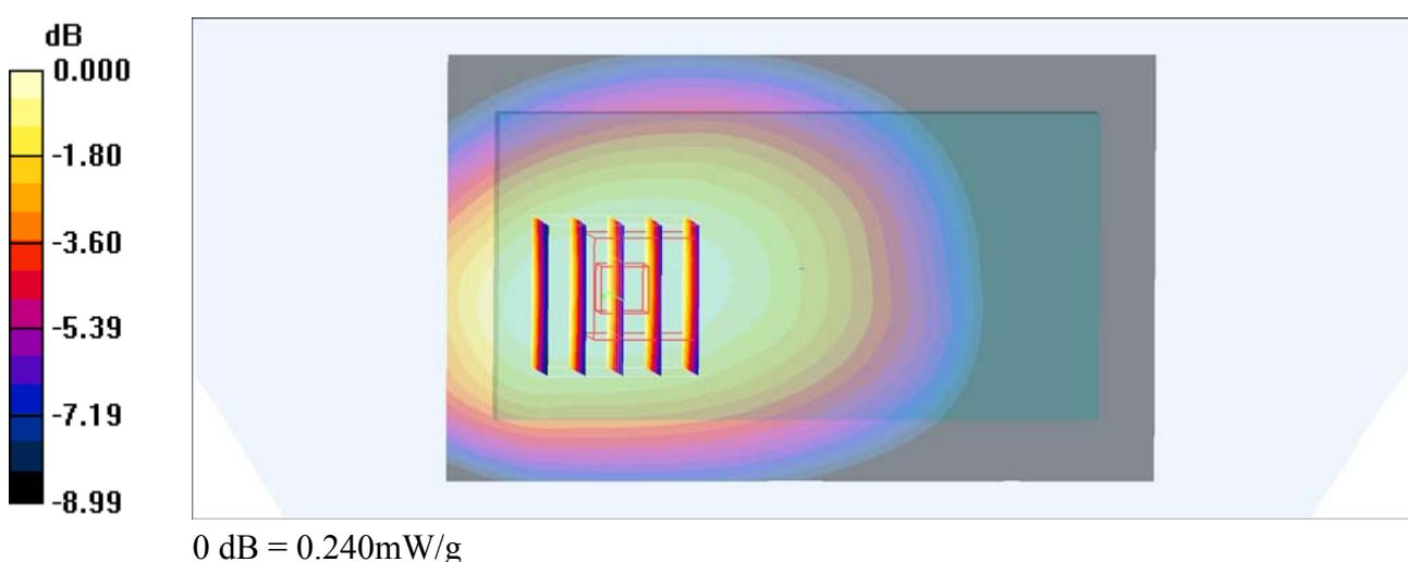
**#29\_LTE Band 5\_10M\_QPSK\_1RB\_0offset\_Back\_15mm\_Ch20450**
