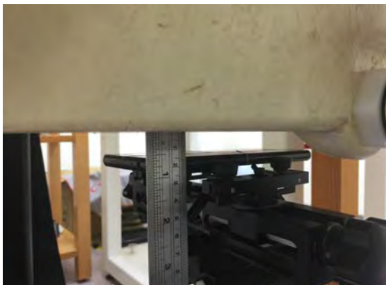
Fig.7 EUT front side to flat phantom
