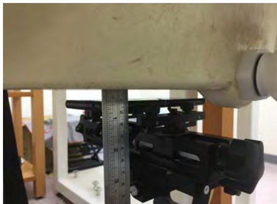
Fig.9 EUT front to flat phantom
