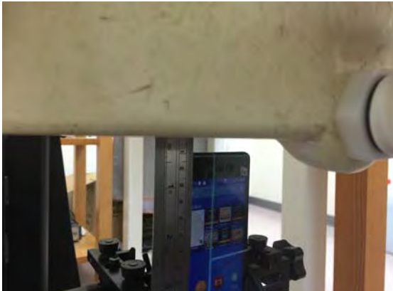
Fig.12 EUT top to flat phantom
