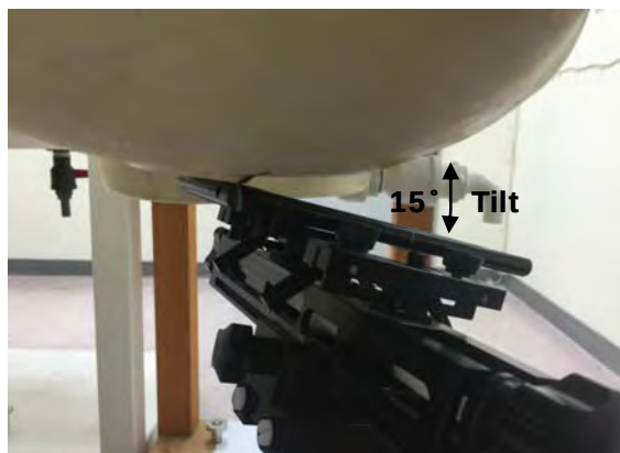
Fig.4 Right Head Section / Ear-Tilt Position(15°)
