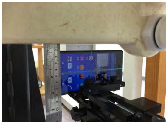
Fig.15 EUT left to flat phantom
