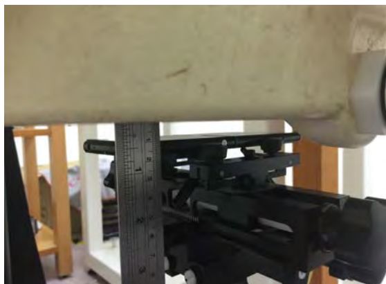
Fig.10 EUT back to flat phantom
