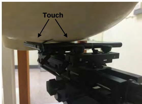
Fig.3 Right Head Section / Cheek-Touch Position
