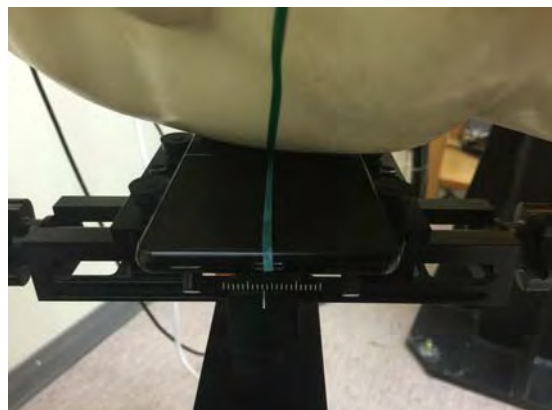
Fig.3 Right Head Section / Cheek-Touch Position
