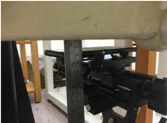
Fig.8 EUT back side to flat phantom
