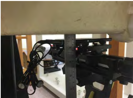
Fig.11 back side with headset to flat phantom
