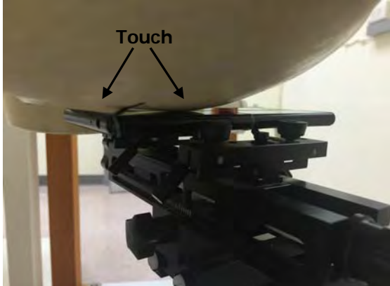
Fig.3 Right Head Section / Cheek-Touch Position
