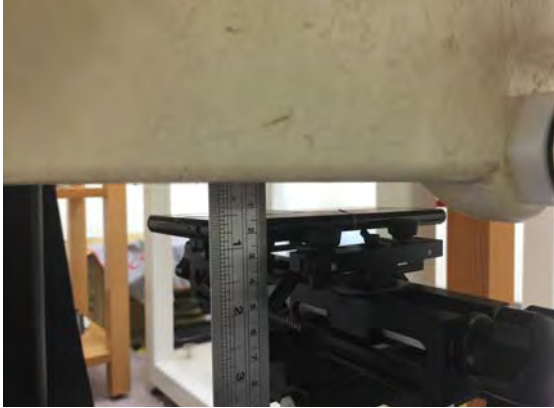
Fig.7 EUT front side to flat phantom
