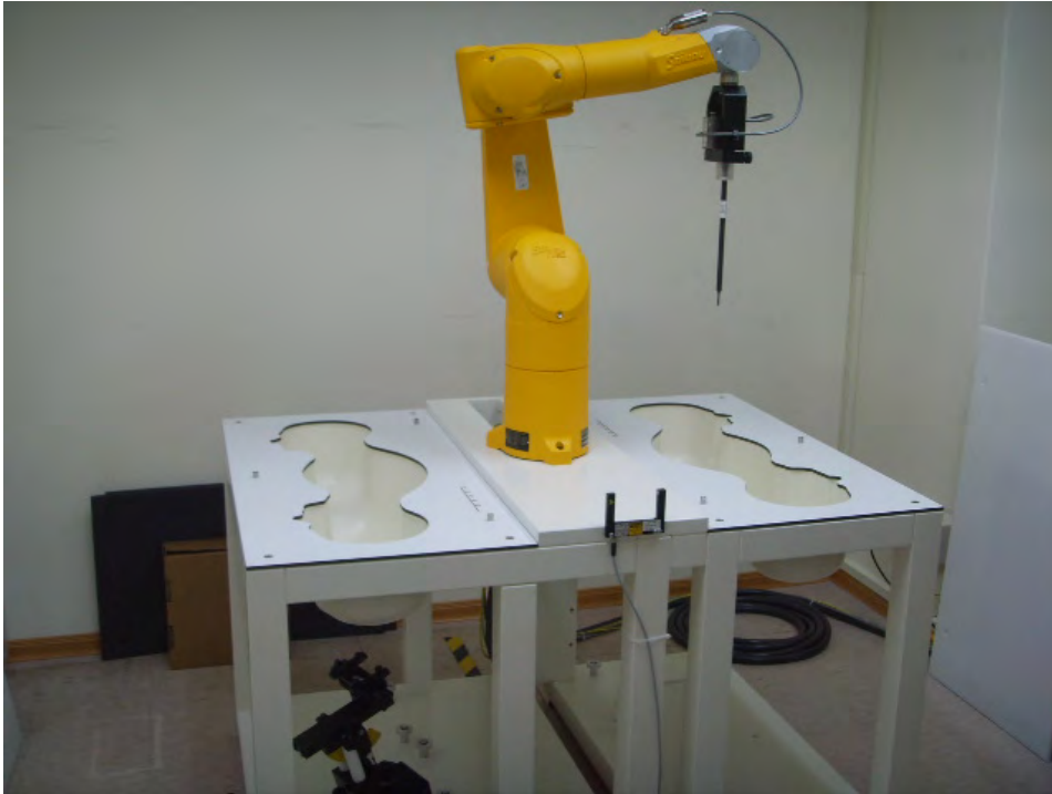
Fig.1 Photograph of the SAR measurement system
