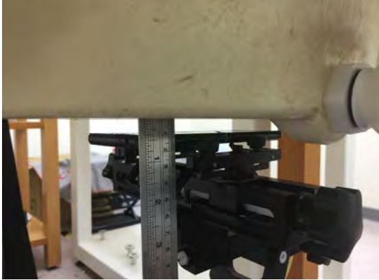
Fig.9 EUT front to flat phantom
