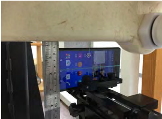
Fig.15 EUT left to flat phantom
