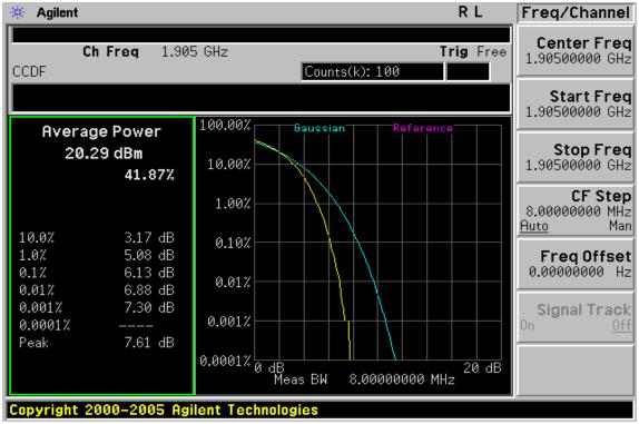
15MHz BW LTE-Band 2(16QAM Number: 75 Offset: 0) Channel Low
