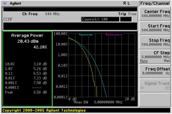
5MHz BW LTE-Band 7(16QAM Number: 25 Offset: 0) Channel Low
