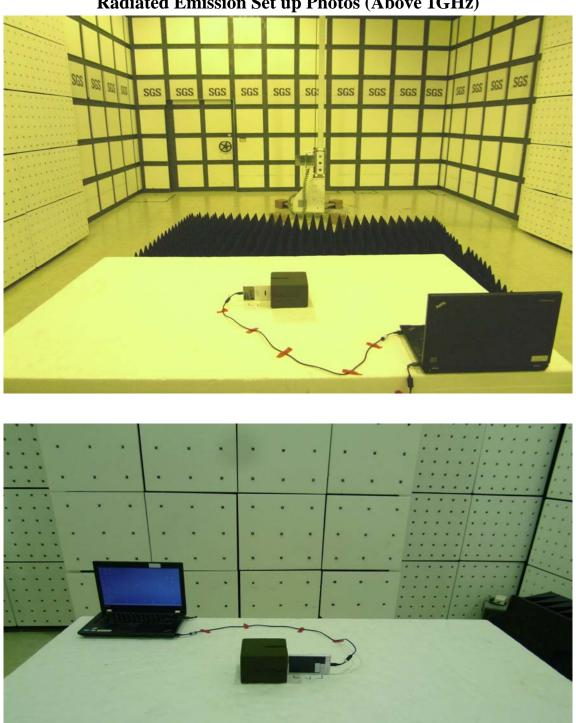
**Radiated Emission Set up Photos (Above 1GHz)**
