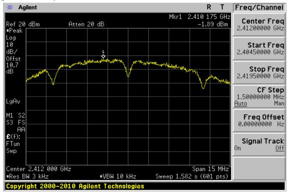
**Power Spectral Density Test Plot (CH-Mid)**
