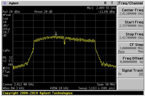
**Power Spectral Density Test Plot (CH-Mid)**
