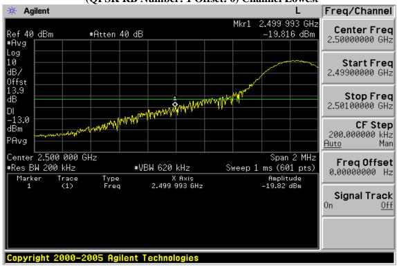
Band edge emission at antenna terminals –15MHz BW LTE-Band 7 (QPSK RB Number: 1 Offset: 74) Channel Highest
