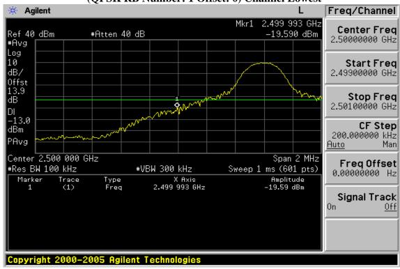
Band edge emission at antenna terminals –10MHz BW LTE-Band 7 (QPSK RB Number: 1 Offset: 49) Channel Highest
