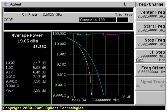
5MHz BW LTE-Band 7(16QAM Number: 25 Offset: 0) Channel Mid
