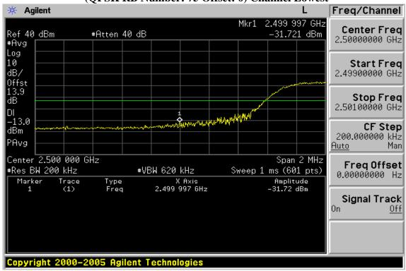
Band edge emission at antenna terminals –15MHz BW LTE-Band 7 (QPSK RB Number: 75 Offset: 0) Channel Highest
