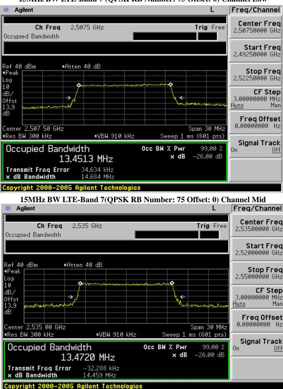
15MHz BW LTE-Band 7 (OPSK RB Number: 75 Offset: 0) Channel Low
