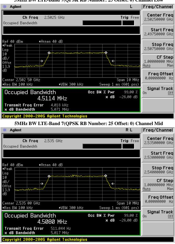
5MHz BW LTE-Band 7(QPSK RB Number: 25 Offset: 0) Channel Low
