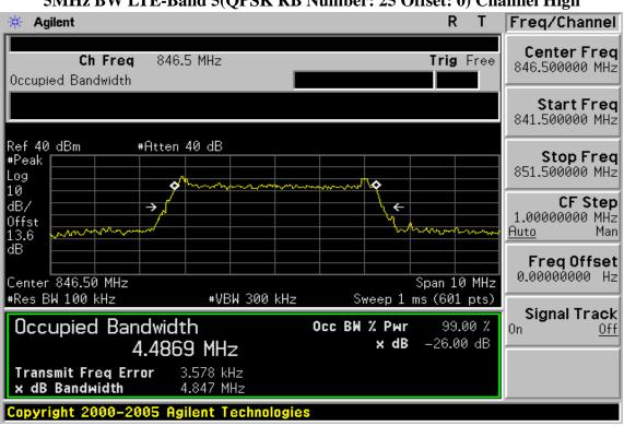
5MHz BW LTE-Band 5(QPSK RB Number: 25 Offset: 0) Channel High
