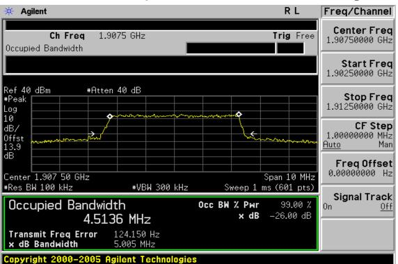
5MHz BW LTE-Band 2(QPSK RB Number: 25 Offset: 0) Channel High
