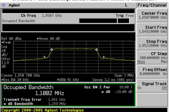
1.4MHz BW LTE-Band 2(QPSK RB Number: 6 Offset: 0) Channel Low
