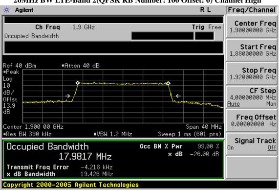
20MHz BW LTE-Band 2(QPSK RB Number: 100 Offset: 0) Channel High
