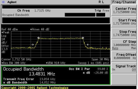
15MHz BW LTE-Band 4(16QAM RB Number: 75 Offset: 0) Channel High
