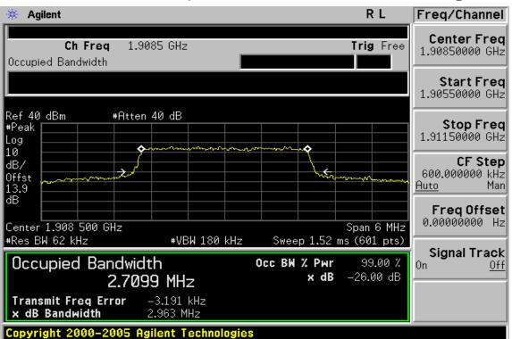
3MHz BW LTE-Band 2(QPSK RB Number: 15 Offset: 0) Channel High
