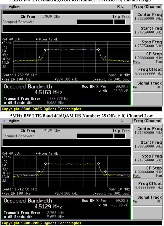
5MHz BW LTE-Band 4(QPSK RB Number: 25 Offset: 0) Channel High
