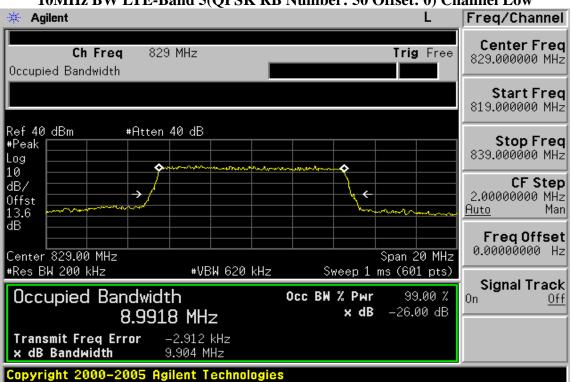
10MHz BW LTE-Band 5(QPSK RB Number: 50 Offset: 0) Channel Low
