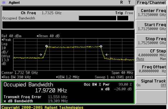
20MHz BW LTE-Band 4(16QAM RB Number: 100 Offset: 0) Channel High
