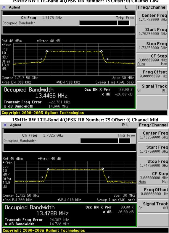
15MHz BW LTE-Band 4(QPSK RB Number: 75 Offset: 0) Channel Low
