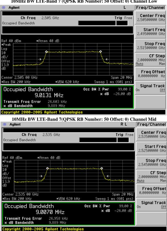
10MHz BW LTE-Band 7 (OPSK RB Number: 50 Offset: 0) Channel Low
