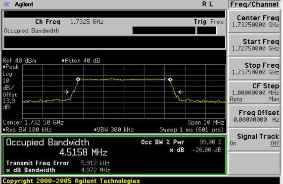
5MHz BW LTE-Band 4(16QAM RB Number: 25 Offset: 0) Channel High
