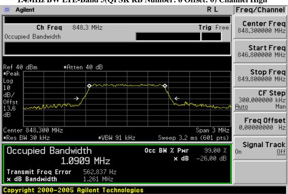
1.4MHz BW LTE-Band 5(QPSK RB Number: 6 Offset: 0) Channel High
