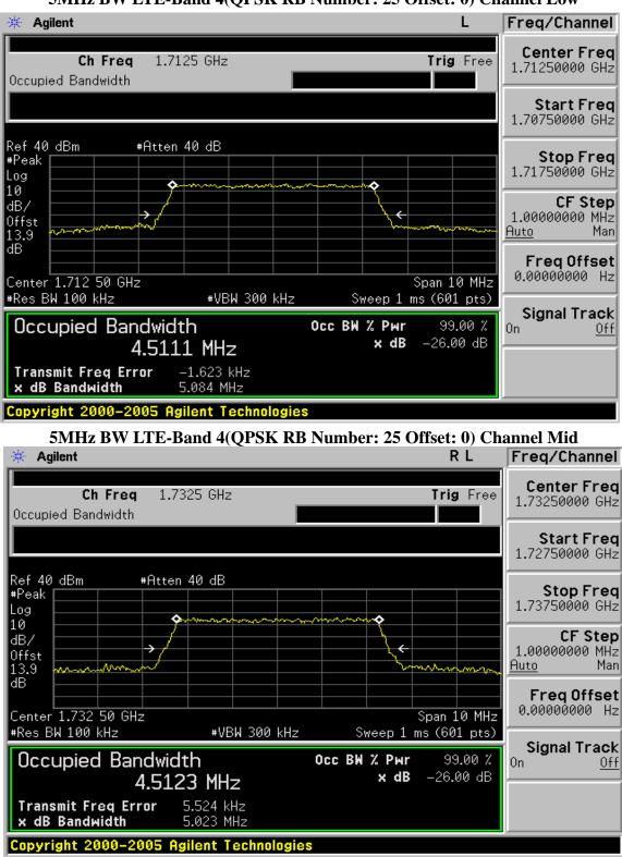
5MHz BW LTE-Band 4(QPSK RB Number: 25 Offset: 0) Channel Low
