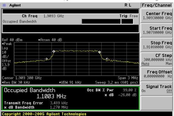
1.4MHz BW LTE-Band 2(QPSK RB Number: 6 Offset: 0) Channel High
