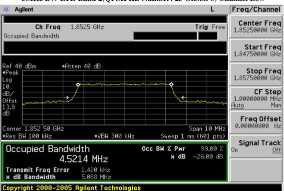
5MHz BW LTE-Band 2(QPSK RB Number: 25 Offset: 0) Channel Low
