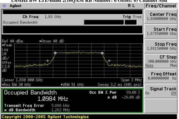
1.4MHz BW LTE-Band 2(16QAM RB Number: 6 Offset: 0) Channel Mid
