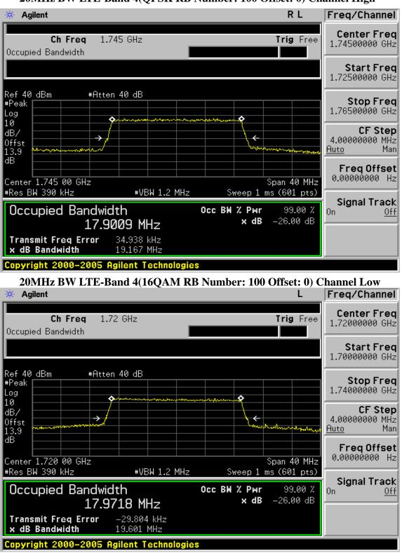
20MHz BW LTE-Band 4(QPSK RB Number: 100 Offset: 0) Channel High
