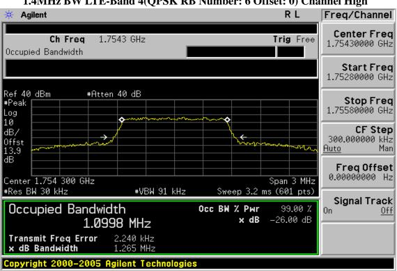
1.4MHz BW LTE-Band 4(QPSK RB Number: 6 Offset: 0) Channel High
