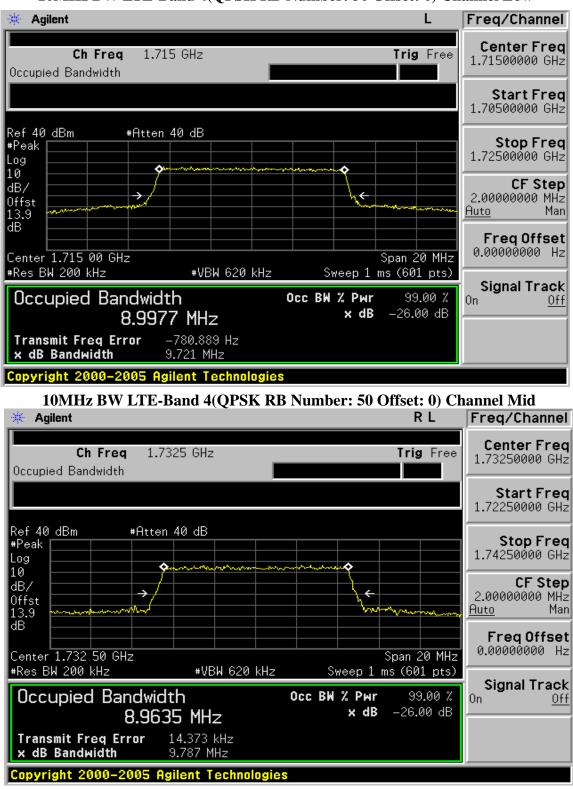
10MHz BW LTE-Band 4(OPSK RB Number: 50 Offset: 0) Channel Low
