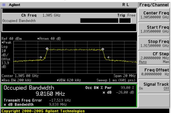
10MHz BW LTE-Band 2 (QPSK RB Number: 50 Offset: 0) Channel High
