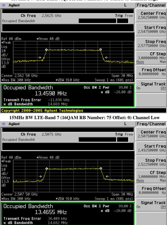
15MHz BW LTE-Band 7(QPSK RB Number: 75 Offset: 0) Channel High
