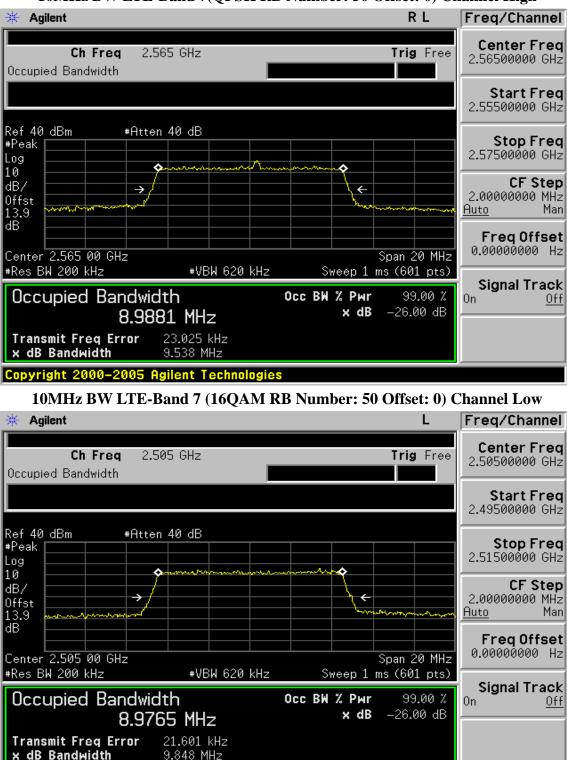
10MHz BW LTE-Band 7(QPSK RB Number: 50 Offset: 0) Channel High
