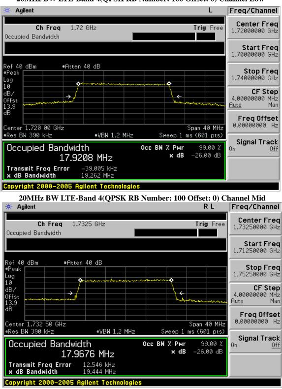
20MHz BW LTE-Band 4(OPSK RB Number: 100 Offset: 0) Channel Low
