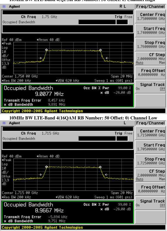
10MHz BW LTE-Band 4(QPSK RB Number: 50 Offset: 0) Channel High
