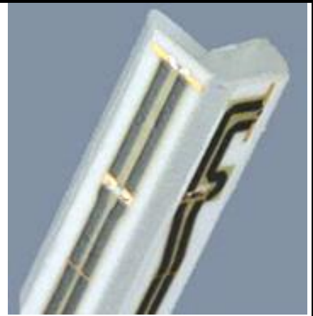
Fig 5.2 Photo of E-field Probe
