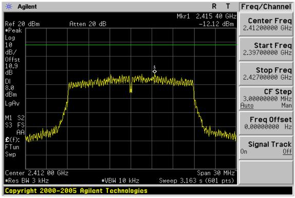
**Power Spectral Density Test Plot (CH-Mid)**
