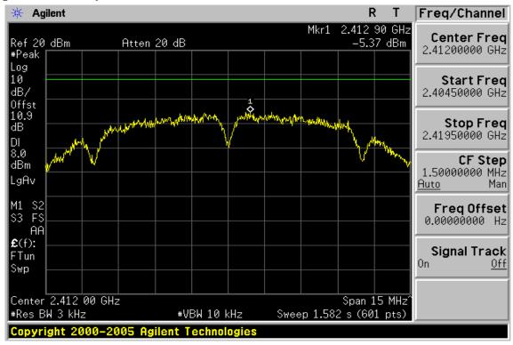
**Power Spectral Density Test Plot (CH-Mid)**
