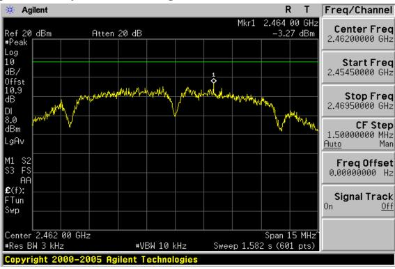
802.11g **Power Spectral Density Test Plot (CH-Low)**
