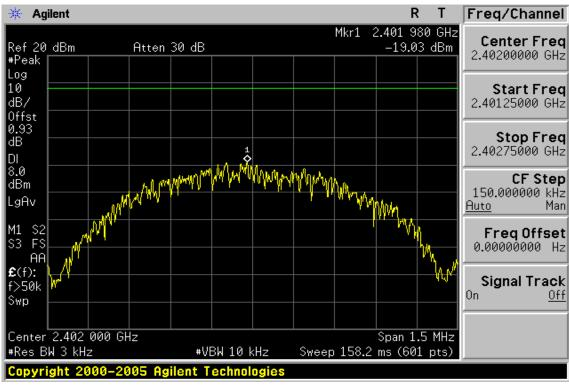
**Power Spectral Density Test Plot (CH-Mid)**
