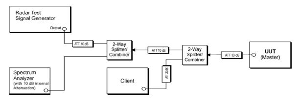
Setup for Client with injection at the Master
