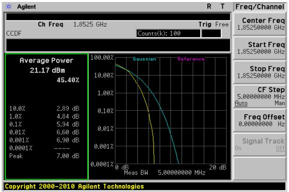
Figure 13-53: 5MHz BW LTE-Band 2(16OAM Number: 25 Offset: 0) Channel Mid
