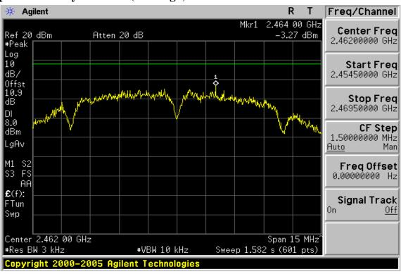
802.11g **Power Spectral Density Test Plot (CH-Low)**
