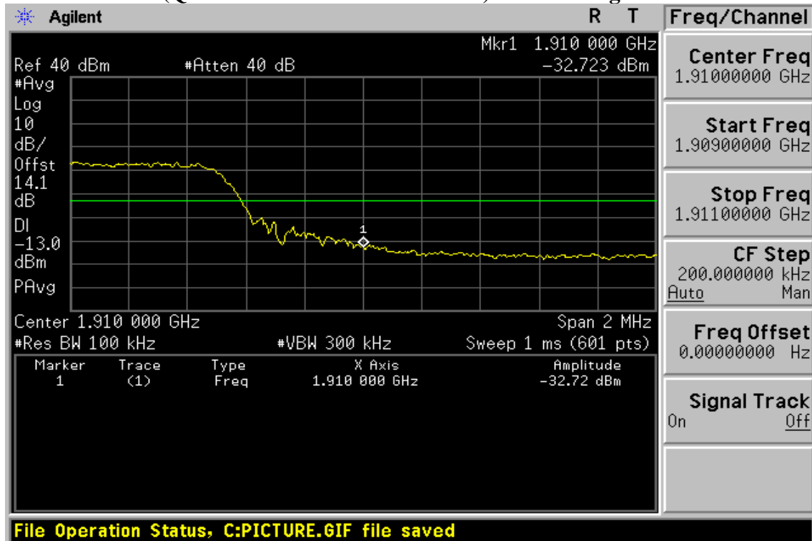
Figure 9-103: Band edge emission at antenna terminals –10MHz BW LTE-Band 2 (QPSK RB Number: 50 Offset: 0) Channel Highest
