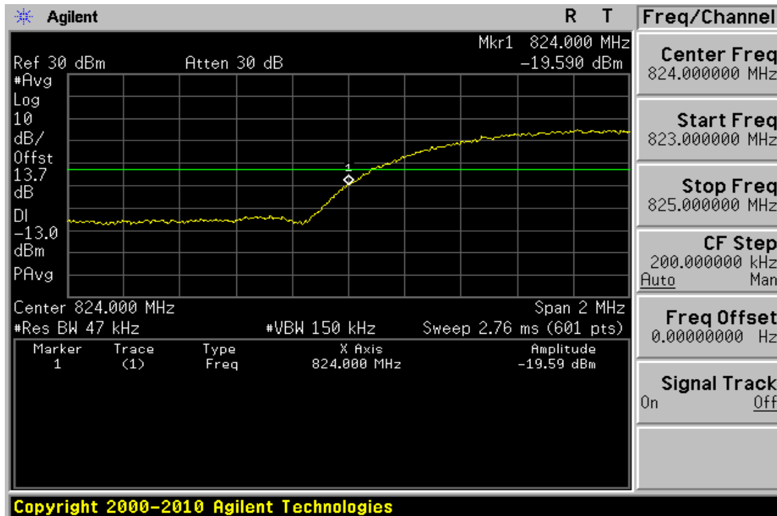
Figure 9-40: Band edge emission at antenna terminals – WCDMA V Channel Highest
