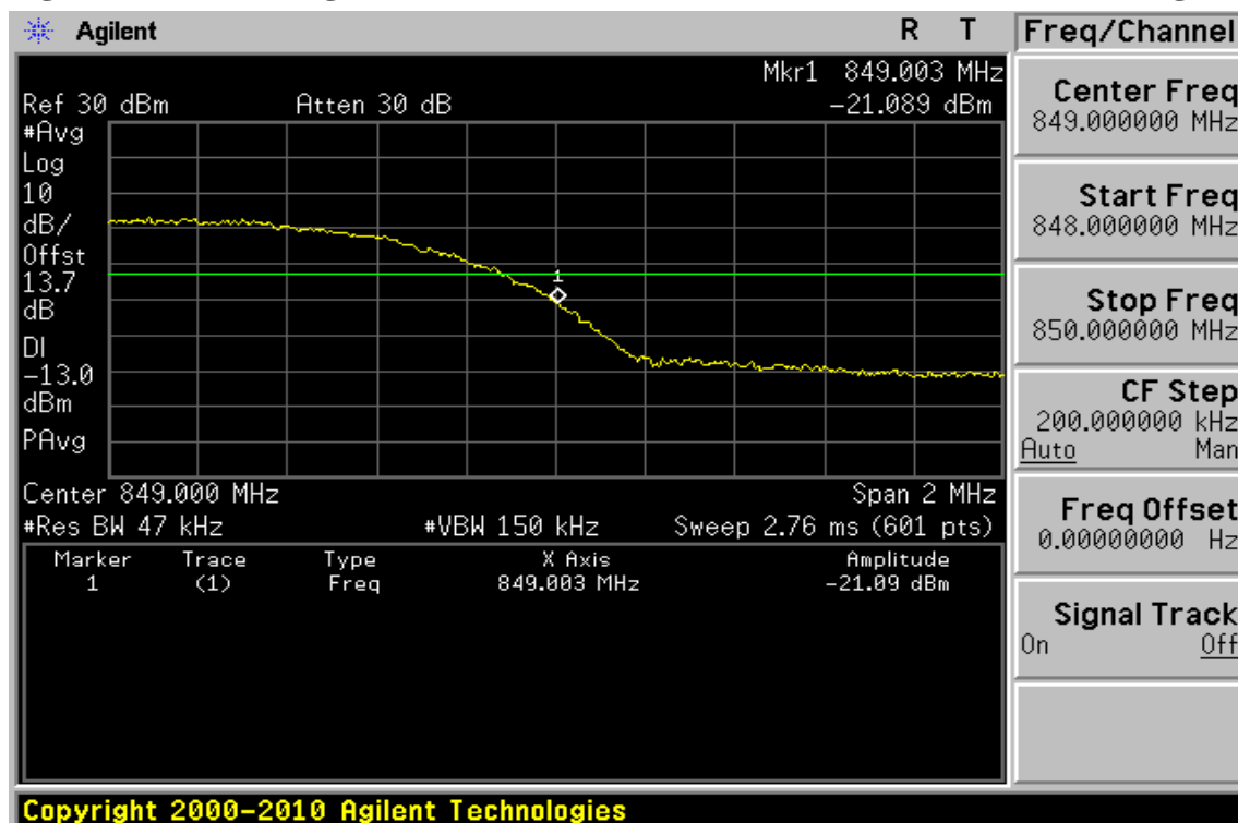
Figure 9-50: Band edge emission at antenna terminals – HSDPA V Channel Highest
