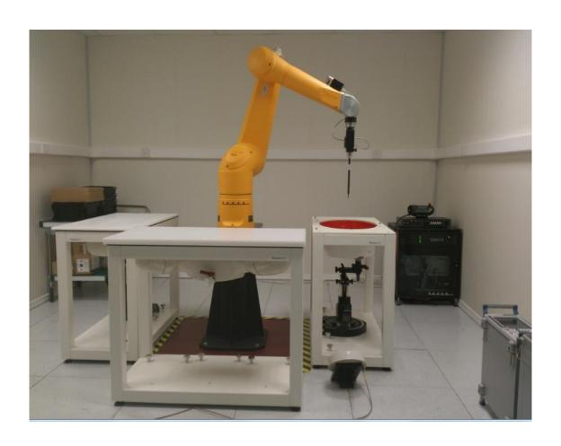
Picture 1: Specific Absorption Rate Test Layout
